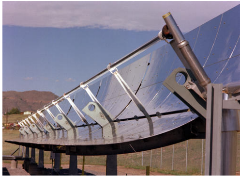
Figure 58. Parabolic Trough Collector
