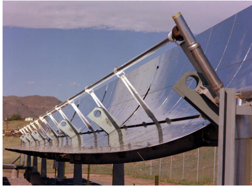
Figure 8. Parabolic Trough Collector
